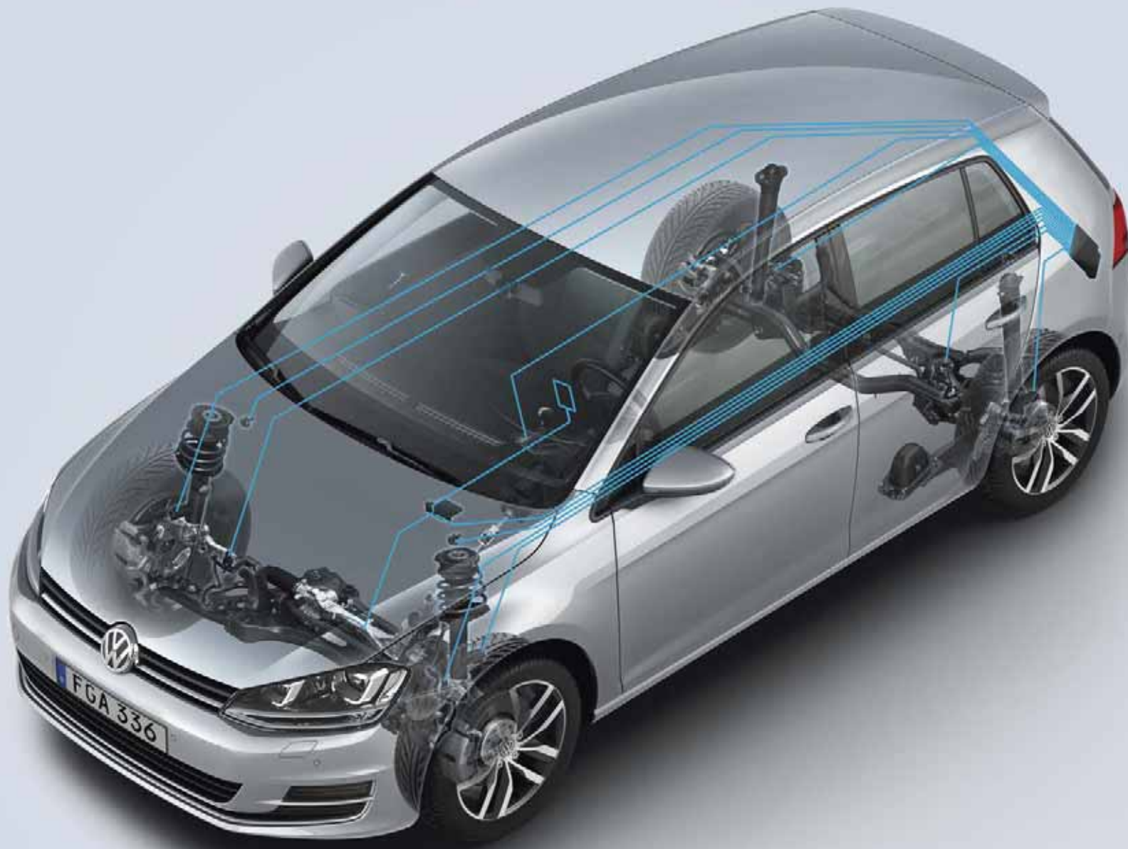
DCC, Dynamic Chassis Control
